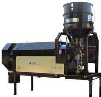
New for the 2013 season Court Seeds has added a second seed treater to increase our treating capacity. This new treater is specifically designed for soybeans and features a mixing drum to ensure even distribution of seed treatments and gentler handling of seeds. Additionally, we will be able to apply both seed
